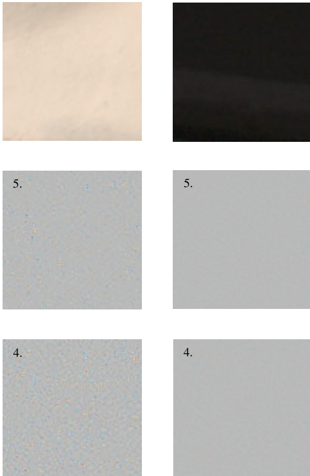
Fig. 8: Compression noise structure of model 1 (configurations 4. and 5. of tab. 1) for bright (left column) and dark (right column) areas. The deviations
